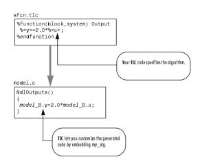
The S-function timestwo.c provides a simple example of a fully inlined S-function. This block multiplies its input by 2 and outputs it. The C-MEX version of the block is in matlabroot/simulink/src/timestwo.c, and the inlining TLC file for the block is in matlabroot/toolbox/simulink/blocks/tlc c/timestwo.tlc.
