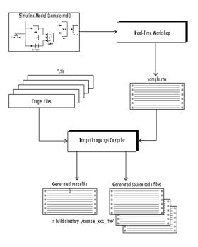
When generating code from a Simulink model using Real-Time Workshop, the first step in the automated process is to generate a *model*.rtw file. The *model*.rtw file includes all the model-specific information required for generating code from the Simulink model. *model*.rtw is passed to the Target Language Compiler, which uses it in combination with a set of included system target files and block target files to generate the code.
