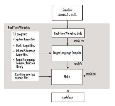
The Target Language Compiler (TLC) is designed for one purpose — to convert the model description file *model*.rtw (or similar files) into target-specific code or text.
