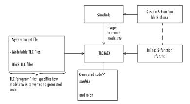
Just as a C program is a collection of ASCII files connected with #include statements and object files linked into one binary, a *TLC program* is a collection of ASCII files, also called *scripts*. Because the Target Language Compiler is an interpreted language, however, there are no object files. The single target file that calls (with the %include directive) all other target files needed for the program is called the *entry point*.
